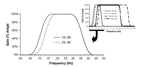
Fig. A.2. Transfer function of filters used by CMetX. Larger panel shows the default .12–.40 Hz bandpass filter and the alternate .15–.40 Hz filter for adults, whereas inset shows all four available filters. All filters are 241-point FIR filters.
